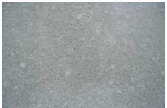
Fig. 5.2 Coarse aggregate imprints itself on the surface
